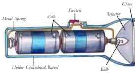
Fig. 7 : Inside view of a torch-light
