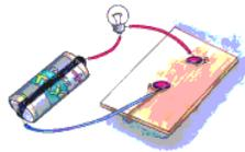
Fig. 8 : An open electric circuit
